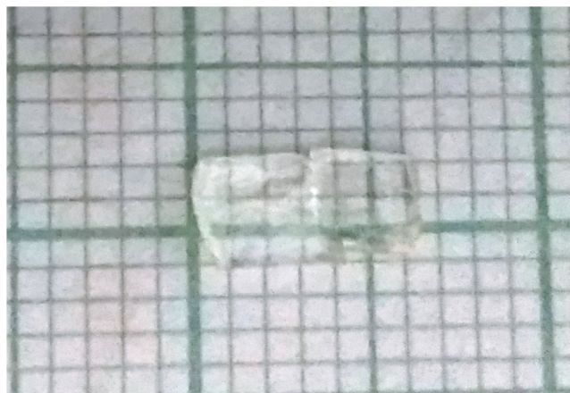
Fig. 1. Grown crystal of PBCPM by solvent evaporation method.
